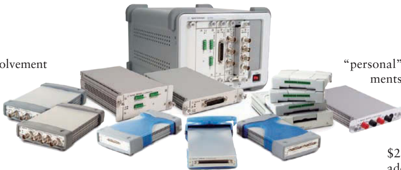
Fig. 3 USB instruments are available in a wide variety of functions, operating as individual units or by plugging into a chassis to form a complete test platform. Courtesy of Agilent Technologies.
