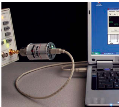
Fig. 2 In addition to DSOs and data-acquisition units, USB instrumentation provides RF and microwave test capabilities such as power meters and synthesized sources.
