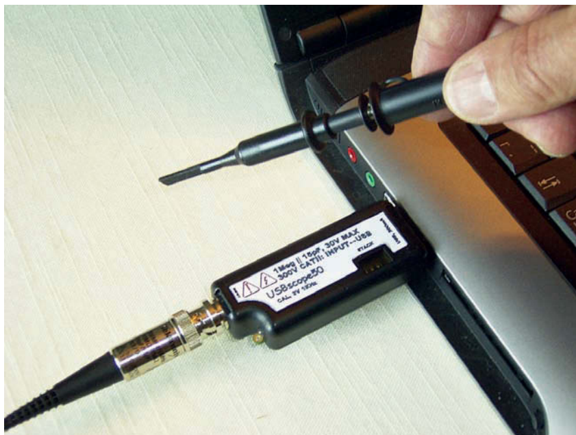
Fig. 1 USB instruments can pack considerable test capability into a tiny package, such as this 50-Msamples/s shirt-pocket digital storage oscilloscope.
